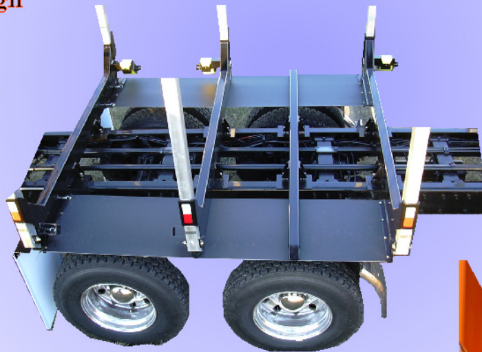
Rubber Belted Fender System with Bucket Frame Guard Protector
