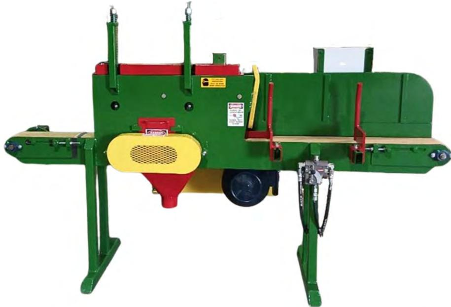
The Morgan Military Notcher manufactured by Sawmill Supplies and Equipment is designed to make a precision notch in boards for banding straps. Equipped with split indexable dato chipping blades. Constructed of heavy gauge steel and square tubing.
