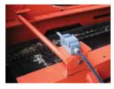
ALL MODELS HAVE SAFETY STOP SWITCHES TO PRE-VENT OVER TRAVEL OF THE WOOD BOX!
