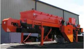
40" Mill, Electric Powered, Stationary, Conveyor Drop
