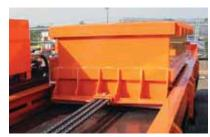
ALL SIZE BOXES ARE CONSTRUCTED OF 1/4" & 1/2" THICK STEEL WALLS AND ARE COM-PLETELY RE-ENFORCED WITH STEEL CHANNEL BEAMS.
