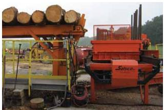
60" Mill, Stationary, 200HP Caterpillar Diesel Engine, **Conveyor Drop**
