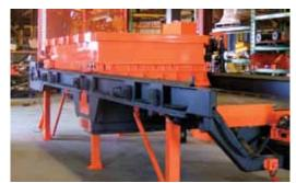
ALL FRAMES ARE CON-STRUCTED OF 8" I-BEAM, CONTINUOUS WELDS & CROSS BEAMS!
