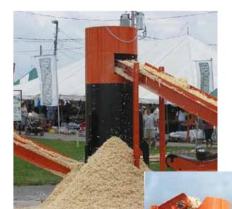
Shavings Conveyor dropped directly from Cutter Shaft, before going through Re-Sizer.
