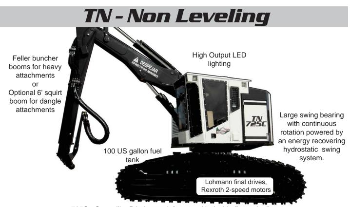
725C - Caterpillar D6 size track frames with double flanged rollers
