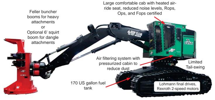
Pictured with TDS22 TimberPro Disc Saw. TBS32 Bar Saw or other attachments available.
