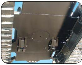
Smooth under-body, with recessed 1" spring-loaded panel allowing easy access for maintenance.
