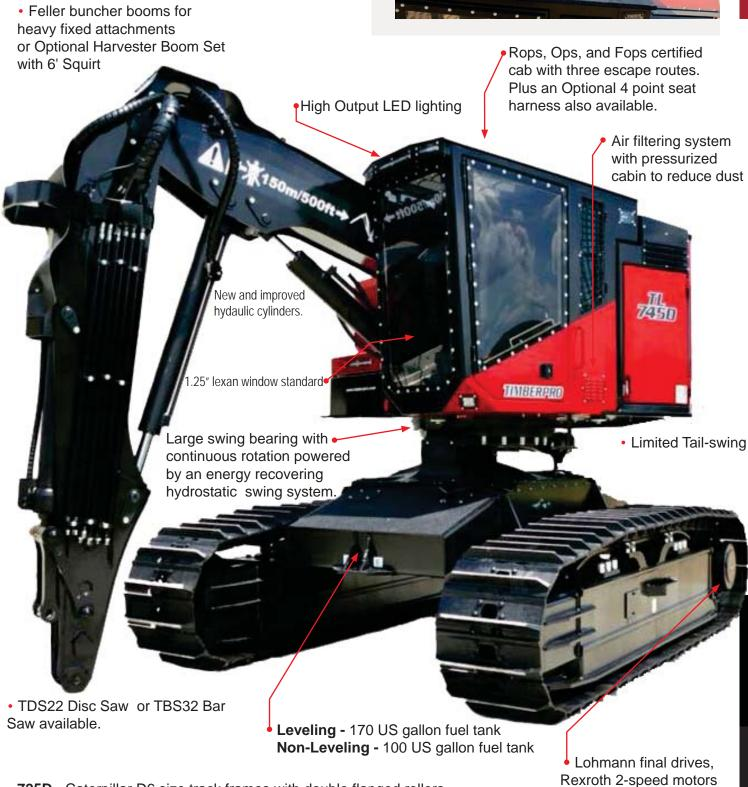
• 735D/745D/755D - Caterpillar D7 size HD track frames with double flanged rollers
