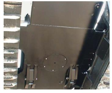
Smooth under-body, with recessed 1" spring-loaded panel allowing easy access for maintenance.
