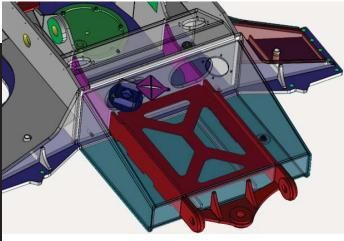
(Optional) Winch Assist / Tethering Hitch available on the 11' 2" Carbody
