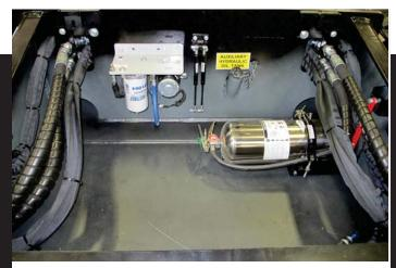
Leveling lower frames feature hydraulic oil storage tank, a new improved Raptor high flow fuel pump and tool storage area.
