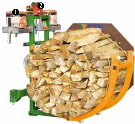
Comfort bundling equipment with Fybron pressed-yarn 1 Dispenser 2 Hand-operated winch
