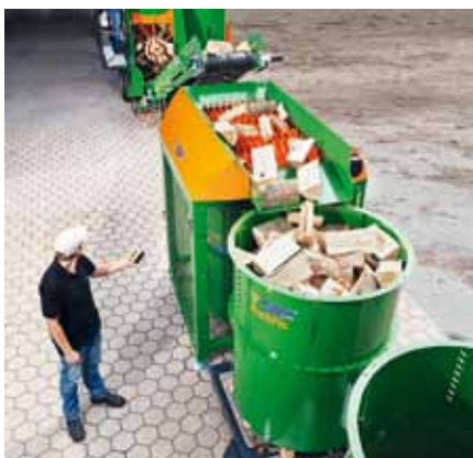
LogFix with optional access guard (Z): High-quality firewood in an instant. Radio remote control for convenient starting and stopping the LogFix.
