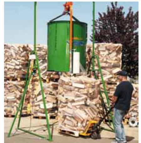
After the filling drum has been fully pulled away towards the top, the finished pack of timber is ready for transport.
