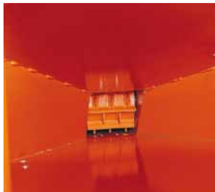
The intake roller takes the material in.
