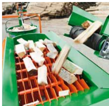
The rotating rollers remove chips and bits of bark from the firewood.
