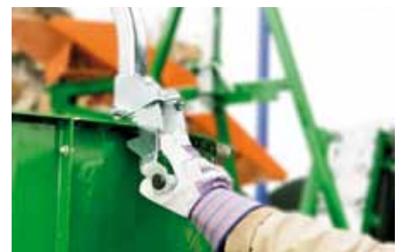
PackFix with quick-change system: It takes but a twist of the hand to detach the filling drum from the frame.
