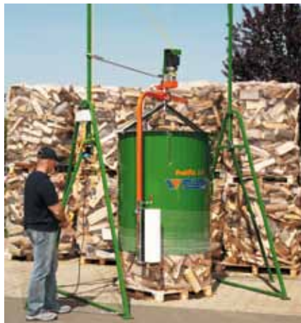
The rotating arm wraps the filling drum with the round bale net.
