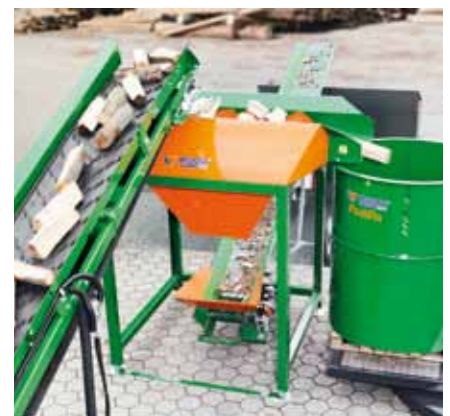
An optional conveyor belt underneath the screen moves the waste to a container. Here, the clean billets fall into a PackFix filling drum.
