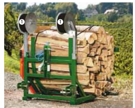
Bundling system with composite band ❶ Dispenser for composite band (M7200 + F0002557 + F0002797).
