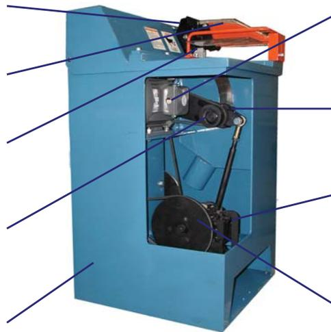
7.5 H.P TEFC Motor is standard 230/460 /3 phase /60 cycle
