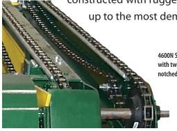
4600N Stackers are configured with two outrigger rails to handle notched stringers.
