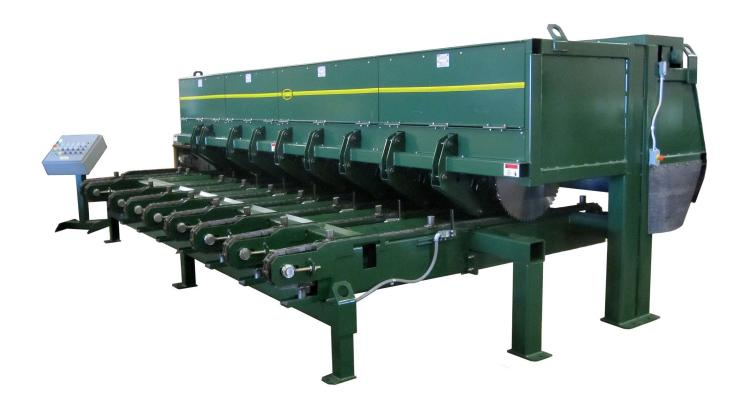
Pendu heavy-duty drop saw trimmers are design-engineered to deliver maximum productivity in mills that end trim and cut boards and cants. Constructed on a rugged, tubular steel frame, each unit is manufactured with powerful 7 1/2HP motors that drive 28" carbide-tipped saw blades. For maximum reliability and long life, all bearings, chains, and sprockets are mounted on flat transfers and powered by 81x chain. Options include bolt on even ending rolls and transfers.
