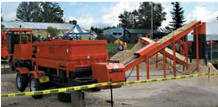
40" Mill, 127HP Caterpillar Diesel Engine, Portable, Conveyor Drop, Shavings Re-Sizer & Conveyors
