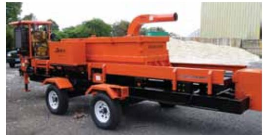
30" Mill, Portable, 91HP Caterpillar Diesel Engine, with Blower
