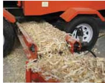
Shavings Conveyor dropped directly from Cutter Shaft, before going through Re-Sizer.
