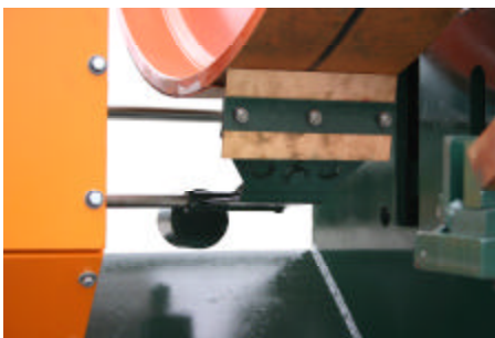
Top wheel scraper tilts and moves up and down with the top wheel.
